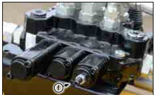
Fig 45 - Valve adjustment, rear of bank
