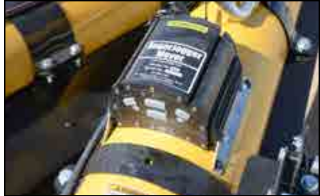
Fig 46 - Electric controls for mover kit
