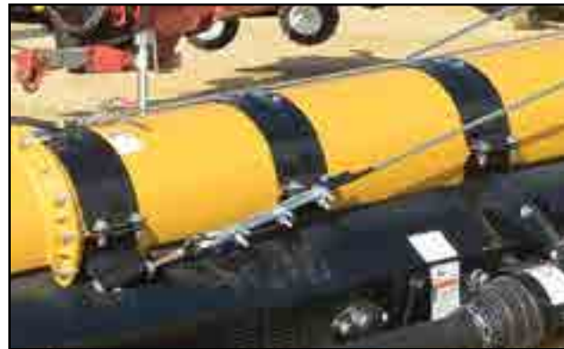
Fig 82 - Eyebolts and cable bridging
