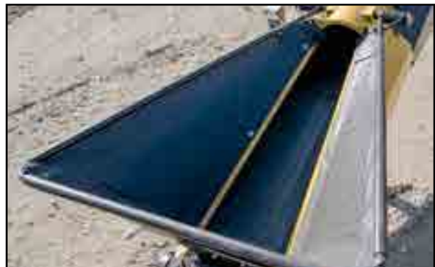
Fig 105 - Completed hopper with belt
