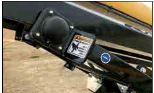
Fig 79 - Upper Lift Bearings
