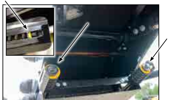
Fig 86 - S-Drive drive box tension bolts w/ tension indicator
