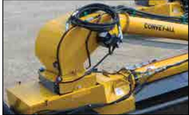
Fig 38 - Swing-out discharge to main conveyor hopper
