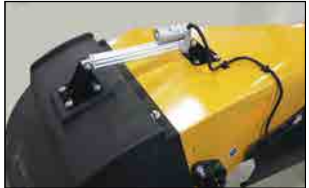
Fig 27 - Discharge spout with electric actuator
