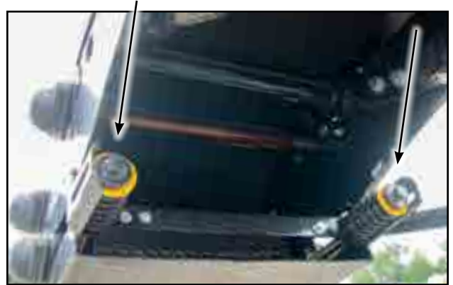
Fig 69 - Tension bolts, Spring Tension Drive Box
