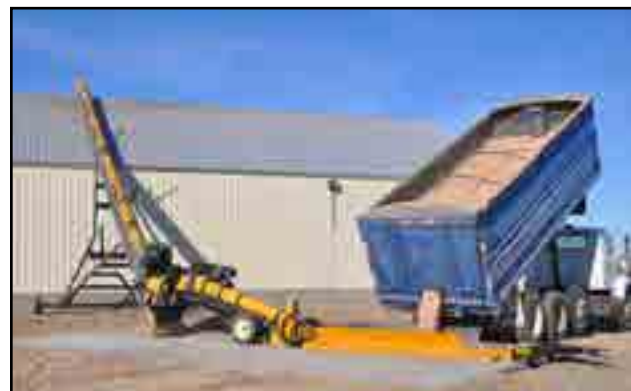
Fig 57 - Drive-over feeding bin fill conveyor
